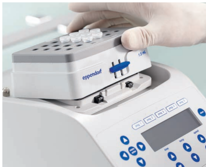
SmartBlock removal from Eppendorf ThermoMixer® C
